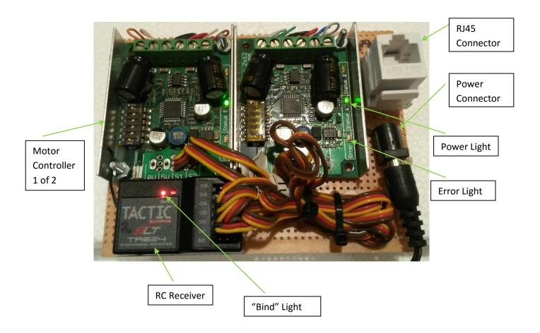
As shown, the motor controller on the left operates the orange and brown motors. The right hand controller operated the blue and green motors.
