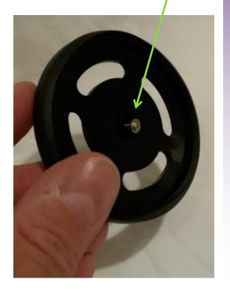
One small line of glue on servo adapter
