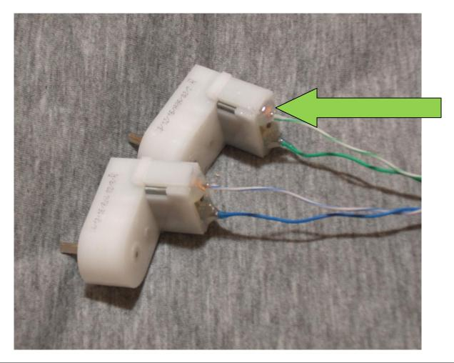
NOTE: It is a good idea to label the motors "right" and "left." The green and green/white wires go to the right motor. The blue and blue/white wires go to the left motor. See sketch below for orientation. It is also good to test the motor assembly when completed. Follow the instructions in the Wired Remote Control document to construct and use a hard wired controller.
