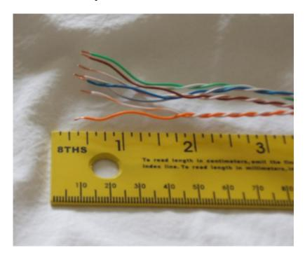
NOTE: The installation of the Molex connectors is only needed if you plan to use these harnesses for the 4 motor Roboxsumo program. Basic Roboxsumo uses only two motors connected to the blue and green wires. The orange and brown wires can be wrapped up or simply cut off if not needed and skip steps 5 and 6. This simplifies and reduces the cost of the harness assembly.
