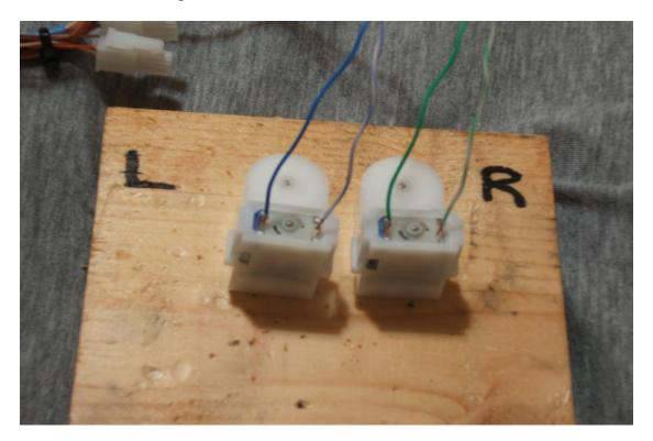
CAUTION: There are small, steel, tabs on the back of the motor near the terminals. Make certain that the wires do not make contact with the steel tabs. This can cause a short during operation. Be careful when soldering the wires in place. Use a medium power (30-40 watt) soldering iron and solder the wire connections quickly to prevent heat damage to the motors.
