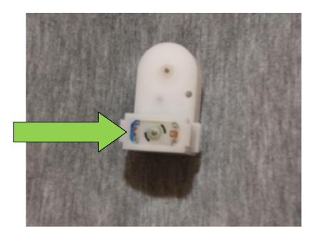
**Step Eight** – In many cases, the motor terminals can be bent or folded when they come out of the packaging. Unfold the terminals very carefully and make sure they are standing straight out of the back of the motor. There should be a small, oval, opening in each of the terminals. Sometimes the utility knife or needle nose pliers can be used to help unfold or straighten the terminals.
