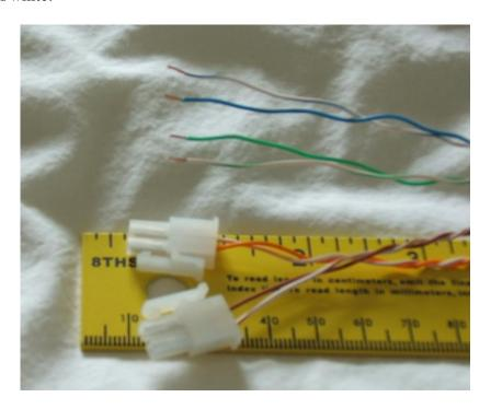
**Step Seven** – At this step you will be attaching the leads to the motor first using solder and then hot glue. If you look closely at the two terminals on the motor, you will see that one of them has a blue mark. This is the terminal that will connect to the solid colored (blue or green) wire. Which motor you attach which wire to is important and is discussed next. The hot glue will be used to provide electrical insulation and strain relief.
