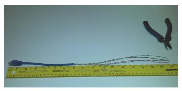
**Step Three** – Splay the ends of the exposed inner cables to spread out the conductors.
