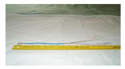
**Step Four** – Strip about 5-8 mm from the ends off all eight of the wires on the 9" exposed section using the wire strippers. Twist the conductors to keep them pulled together in to a tight bundle. This makes them easier to insert in the motors and pins.
