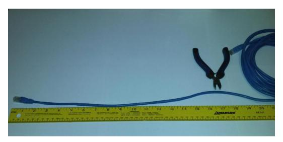
**Step Two** – Use the utility knife to remove approximately  $9\frac{1}{2}$  " of insulation (blue in this case) from the end that does not have the RJ45 molded connector. Leave a 7" strip of insulation on the cable.
