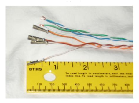
**Step Six** – Attach a Molex connector to the end of the wires that have the pins. Orange and orange/white go to one connector, brown and brown/white to the other. At this point the wiring has been set up so that the solid wires, orange and brown, should be next to the clip and the same with the brown and brown/white.
