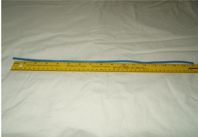
**Step Two** – Use the utility knife to remove approximately 1” of the outer insulation (blue in this case) from one end and 9 ½” from the other end. Leave a 7” strip of insulation on the cable.
